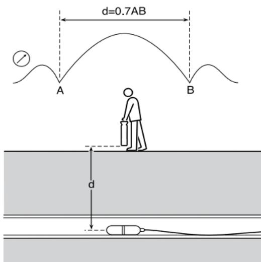
If the signal is too weak or unstable the Receiver unit will not calculate depth. In this case use a more powerful Sonde or use the Pinpoint procedure described below.
