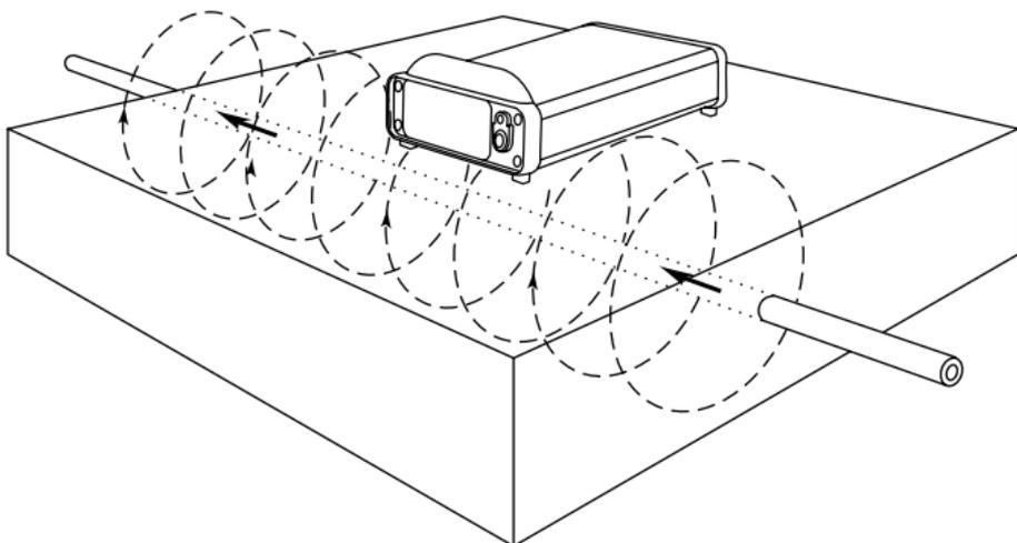
**Note:** Induction cannot apply a signal to a line below reinforced concrete.
