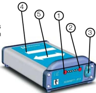
**4** Batteries Access Panel. No tone indicates that the batteries must be replaced. Unscrew fastener on the rear panel and replace with 4 LR20 (D cells) batteries. Observe correct battery polarity as indicated on the top-panel label.
