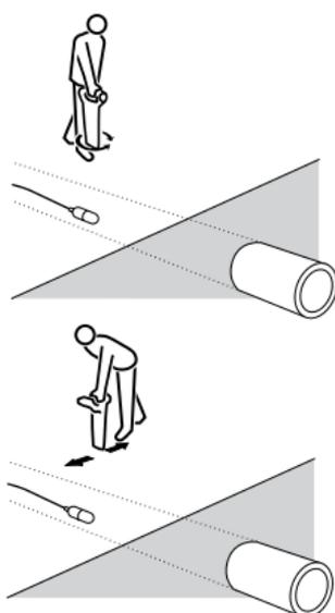
Repeat each step in smaller increments with the Receiver blade resting on or near the ground. The Receiver should now be directly above the Sonde with the blade in line with the Sonde; mark this position.
