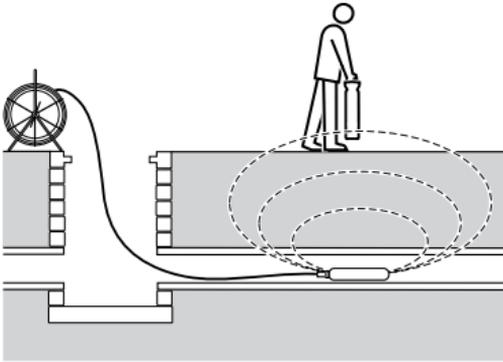
A Sonde radiates a peak field from the center of its axis with ghost signals at each side of the peak. Move the Receiver to one side and then along the axis of the Sonde forwards and backwards to detect the ghost signals.
